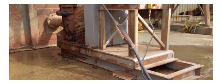
Slurry pumps are mostly large in size and notoriously difficult when it comes to undertaking maintenance and repair. It is a task that usually requires more than one person, the use of lifting aids and one that poses the danger of possible injury to those undertaking the operation.
